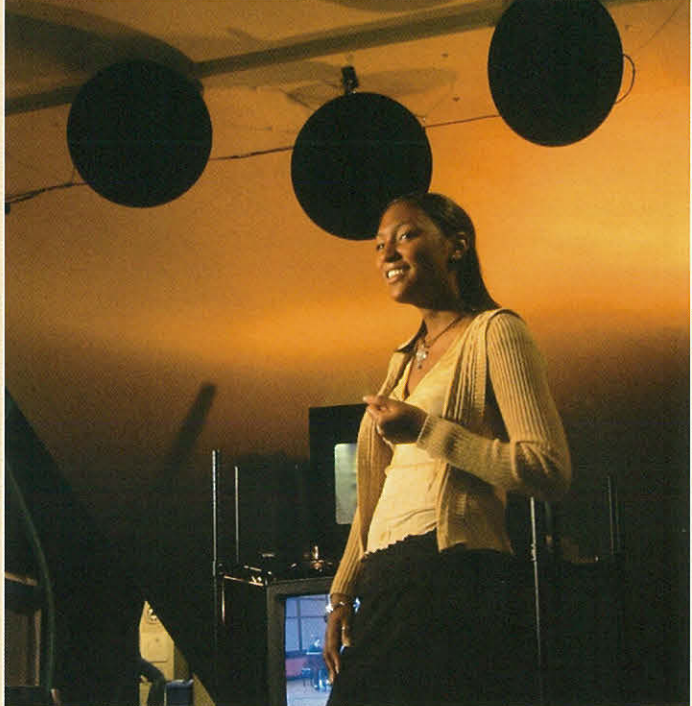
Audio Spotlight represents the first radical departure from traditional loudspeaker technology. The sound is generated in the air itself, indirectly, as a conversion by-product of the interaction of silent ultrasonic waves.
